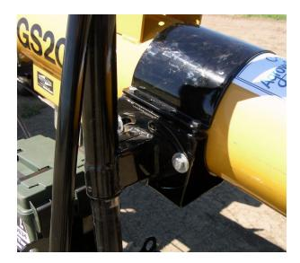
Clamps are available for 8",10", 12", 13", and 14" tubes Clamps can be over slung but give the best clearance under slung Lower the auger and retract the jack when moving the auger with the Back Saver 2
