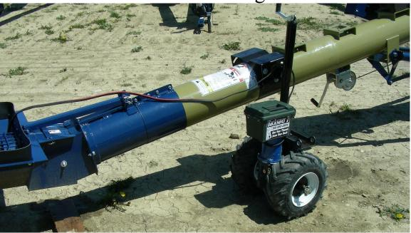
The Back Saver 2 can be used to move truck augers and belt conveyors that have at least 100 pounds of tongue weight. 12 volt remote control uses power from a 12 volt battery. Stays attached for road transport.
