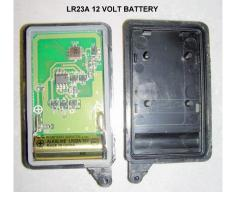
To replace a battery in a key fob pry the back off with a table knife Replace with LR23A 12 volt battery. All key fobs will need to be relearned after replacing a battery
