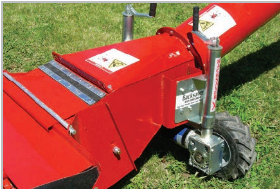
Pictured is the control box that receives the signal from the remote key fobs
