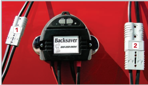
Pictured is the control box that receives the signal from the remote key fobs
